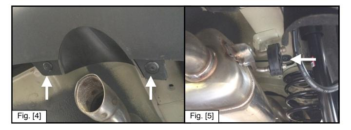
Step 3. Raise the hitch into position by lining up the holes in the hitch frame plates with the weld nuts on the outside of the vehicle frame rails. Thread (1) M10-1.25x40mm hex cap screw, (1) M10 lock washer, and (2) 3/8" flat washer into each of the (4) weld nuts in the frame rails, (2) on the driver and (2) on the passenger sides. Hand tighten all components then be sure that the hitch receiver is level to the vehicle. Once the hitch is level, torque all hardware to 54 ft-lbs. See Figure [6].
